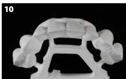
Fig.10: Green state zirconia, before sintering. Thanks to the digitalization, any case is now reproducible.
