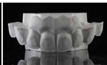
Fig.10: Green state zirconia, before sintering. Thanks to the digitalization, any case is now reproducible.
